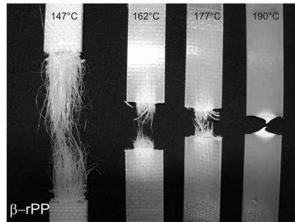
Load-displacement curves and macroscopic failure behavior of all-PP composites 191x168mm (500 x 500 DPI)
