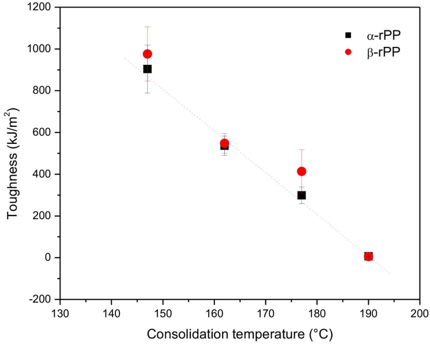
Toughness of the composites as a function of processing temperature
