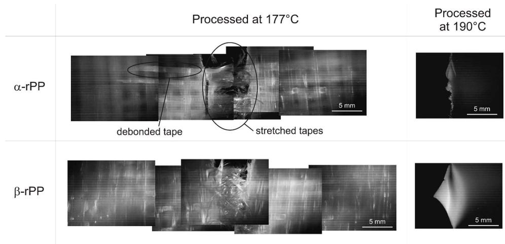
Light microscopy photographs of some typical failures
