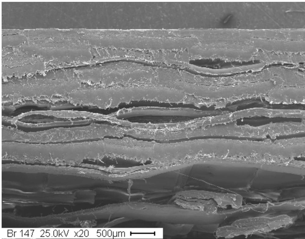
SEM micrograph of typical failure of a poorly consolidated composite
